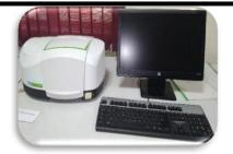
**Fourier Transform Infrared Spectroscopy** (FTIR) relies on the fact that most molecules absorb light in the infra-red region of the electromagnetic spectrum. Any powder and thin film based samples may be characterized to identify the bonding information.
