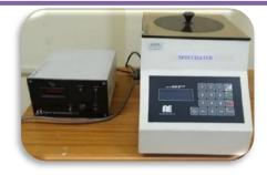
**Spin Coater** is an instrument to deal with coating technology for uniform deposition of thin films on flat substrates. Additionally, heating system is embedded with the same for better adhesion.
