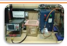
Keithley Source Meter 2450 unit integrated with heating/gas sensing system is used to measure the response of electrical parameters with temperature/gas sensing properties. In addition, an Agilent LCR meter is present to measure the inductance, capacitance and resistance of a circuit.
