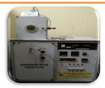
**Magnetron DC Sputtering** is a Deposition technique in which positively charged ions from the plasma are accelerated towards the negatively charged electrode or "target". Any kinds of metals, Cu, Ag, Au, etc. may be deposited on flat substrates using this system.
