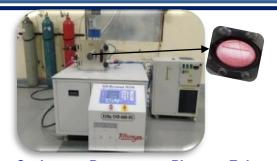
Electron Cyclotron Resonance Plasma Enhanced Chemical Vapour deposition system is used to deposit the high quality thin film using chemical precursor. The equipment is widely used for amorphous Silicon thin film deposition for solar cell, TFT microelectronic applications.
