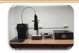
**Solar simulator** provides a controllable indoor test facility under laboratory conditions, used for the testing of solar cells, sun screen, plastics, and other materials and devices.
