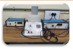
**Two probe** is most commonly used for the measurement of resistivity of very high resistivity samples like sheets/films of polymers. The resistivity measurement of such samples is beyond the range of Four Probe Method.
