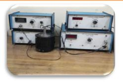
**Four probe** apparatus is one of the standard and most widely used apparatus for the measurement of resistivity of semiconductors.
