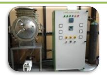
Atmospheric Controller Furnace are designed and manufactured to accommodate wide processing areas where inert atmosphere is required to protect heating samples that are prone to oxidation. Double shell atmosphere furnace with fan cooling; temperature range upto 1200°C.
