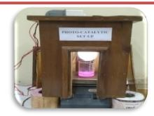
The **Photocatalytic reactor** is used to degrade the organic waste such as dyes, pharmaceutical effluents etc.. The reacting species is stirred by magnetic stirrer.
