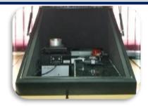
Atomic Force Microscopy (AFM) provides images on the topography of a sample surface by scanning the cantilever over a region of interest. Any solid insulating/conducting film based samples may be characterized.
