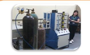
**APCVD setup** is used to produce the desired thin film deposit process on the substrate surface in which the substrate is exposed to one or more volatile precursors, which react and/or decompose on the substrate surface to produce the desired thin film deposit.
