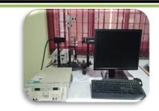
**Contact angle goniometer** using an optical subsystem to capture the profile of a pure liquid on a solid substrate based on the surface wetting behaviour with contact liquid. The angle formed between the liquid–solid interface and the liquid–vapor interface is the contact angle.
